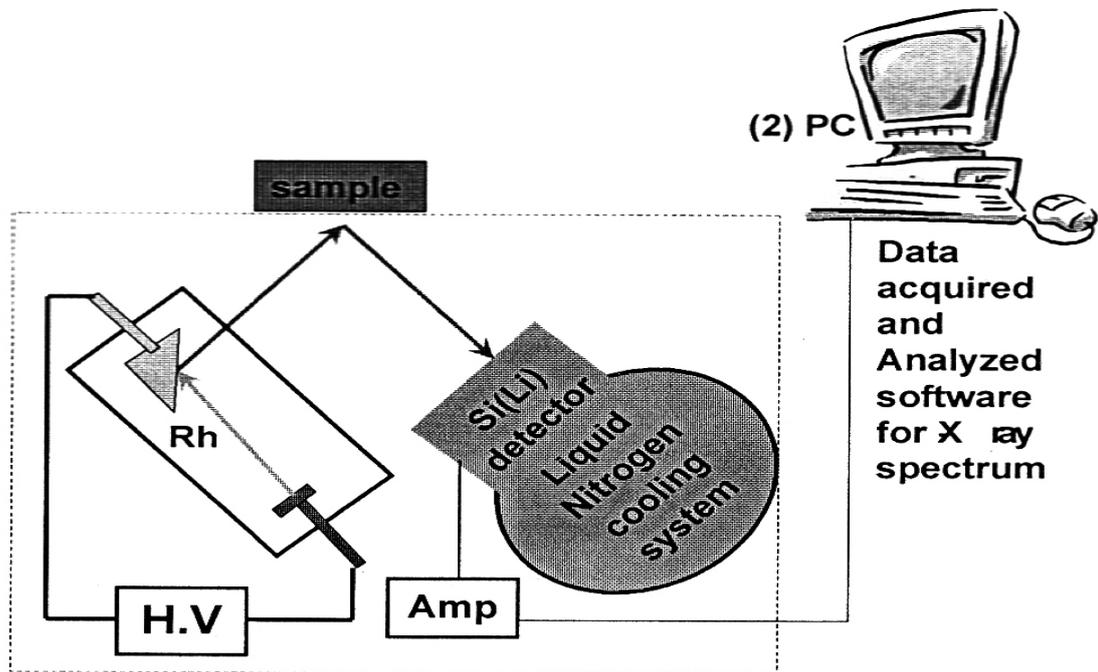
Figure 3(a) Two main parts of the EDX-700 Spectrometer system
